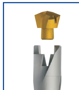
6 Remove Solid Head (Use Gloves to Protect Your Hand From any Danger)
